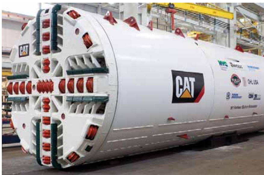
TBM (EPB - mix face)
